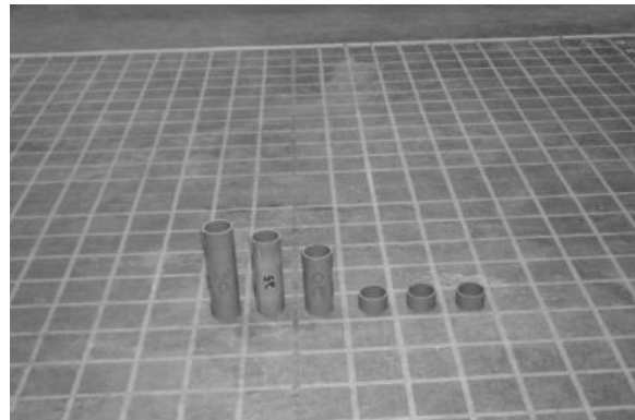
Figure 4. Tubes used to map lower edge of detection zone
