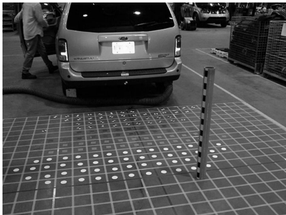
Figure 1. Detection zone test surface and test object.
