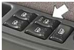
RISKY DESIGNS Horizontal rocker switches (above) and toggle switches (below).
