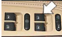
SAFER Lever switches have to be pulled up to raise a car window.
