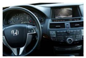
The dashboard of the Honda Crosstour features a rearview camera and monitor that are used when the car is backing up. The function may be required in new cars by 2014. (Genaro Molina / Los Angeles Times)
