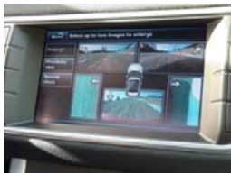
Surround Camera System, in 2012 Land Rover Range Rover Evoque
