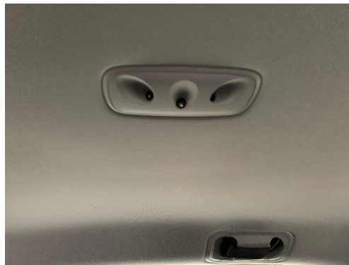
Figure 23. Photo. Hyundai/Kia rear optical sensor.
