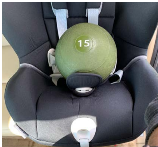
Figure 3. Photo. Sense A Life pad in car seat with 15-lb ball.
