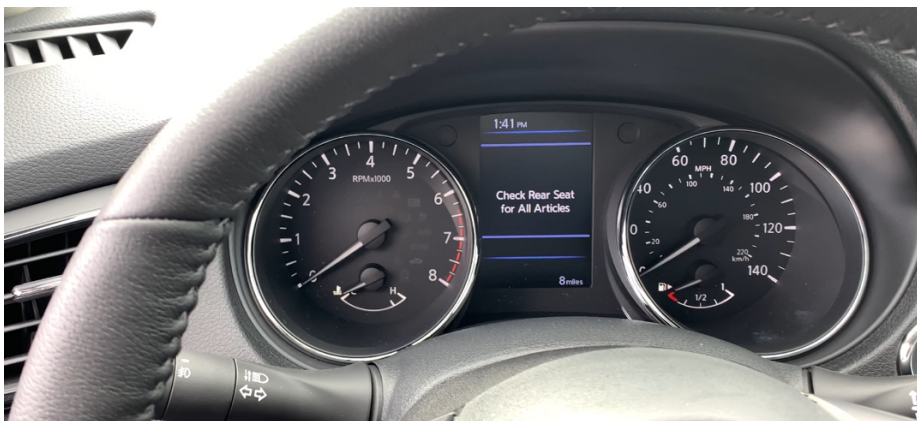
Figure 22. Photo. Nissan Check Rear Seat for All Articles message.
