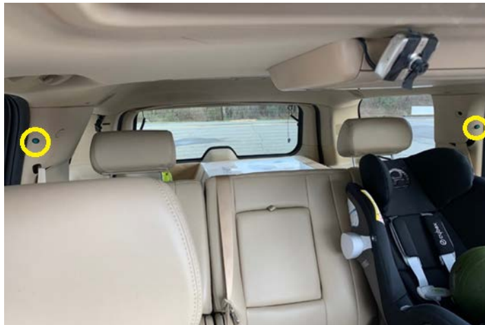
Figure 13. Photo. Ride N Remind buttons in C-pillars.
