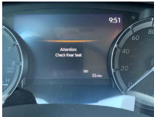
Figure 19. Photo. Toyota RSR Attention: Check Rear Seat message.
