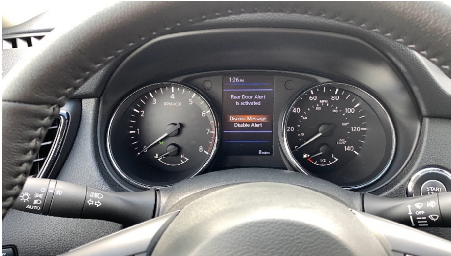
Figure 21. Photo. Nissan RDA is activated message.
