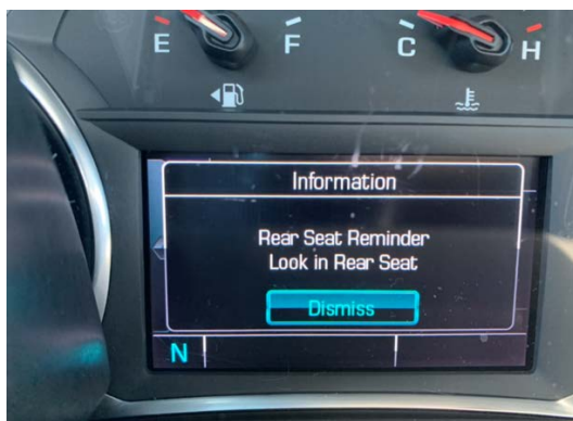
Figure 15. Photo. GM RSR alert.
