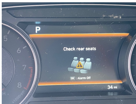
Figure 25. Photo. Hyundai/Kia ROA check rear seats alert.
