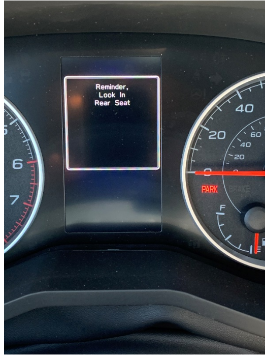
Figure 17. Photo. Subaru RSR Look In Rear Seat message.
