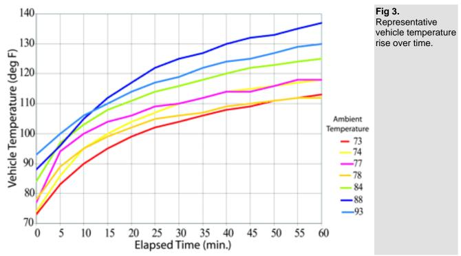
The effect of air conditioning the vehicle before start of measurements was negligible. In preliminary measurements, the vehicle consistently reached ambient temperatures within 5 minutes of the air conditioning's being turning off and then would heat up at a similar rate to non-air-conditioned cases.
