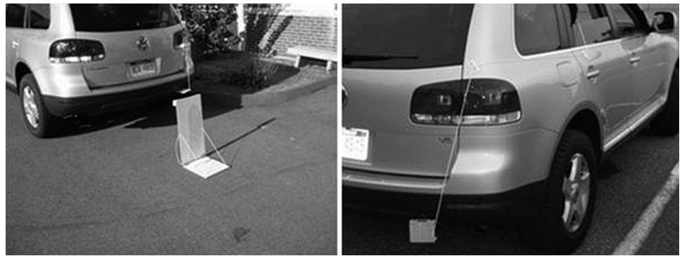
Figure 2 Simulated crash decoy (left), hinged flap for rear audible sensor activation (right).
