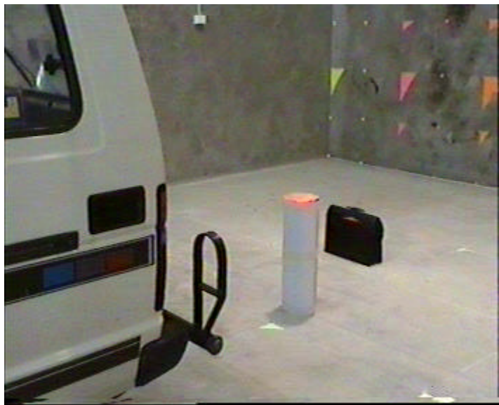
Figure 2b. General view of test layout showing test cylinder (600mm high) and factory wall to rear of vehicle.
