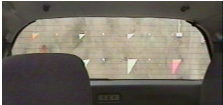
Figure 2a. Example of the view to the rear from driver's seat, showing the marks on the factory wall and rear seat head restraint.
