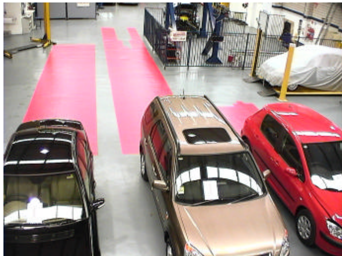
Figure 8. Demonstration of the test results. The red patterns show the area where the 600mm high cylinder would not be visible to an average male driver.
