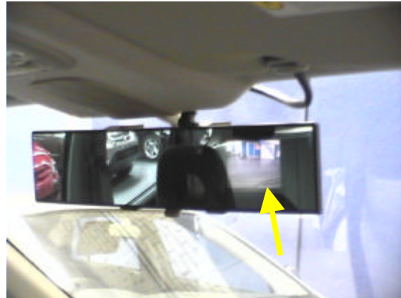
Figure 5. Rear view mirror with built in display screen for rear view camera.
