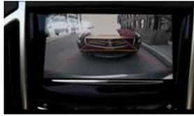
A set of red and yellow guidelines appear on the center stack display, when in reverse, to mark the vehicle's turn radius and allow for easier parking and backing maneuvers. (Photo : General Motors)
