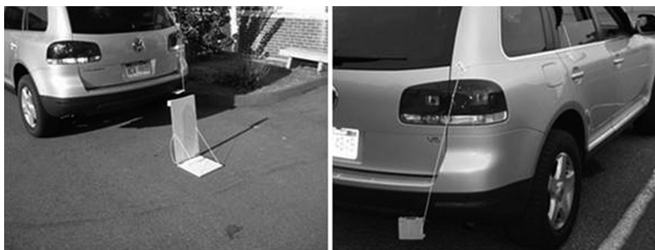
Figure 2 Simulated crash decoy (left), hinged flap for rear audible sensor activation (right).
